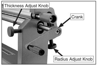
Figure 11. Adjustment knobs (T21324 shown).
